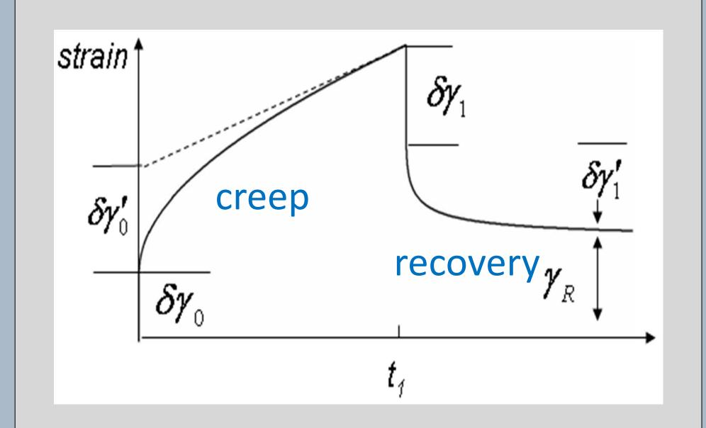
At low stress, the typical ideal creep curve grows monotonically and gradual -ly bends down approaching the steady flow state (constant strain rate) after an instantaneous jump
