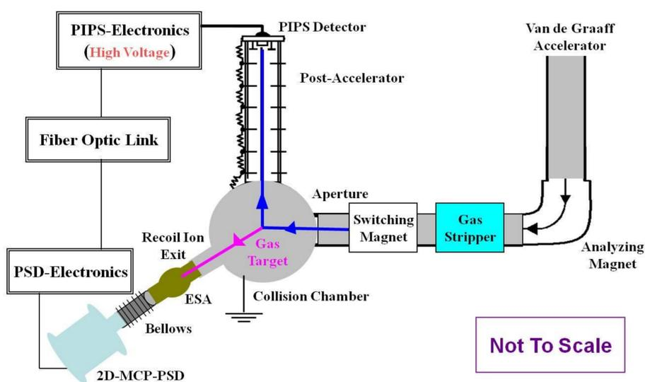
2- The heart of the CRBS experiment is the coincident detection of the backscattered projectile and the recoil target from individual events.
