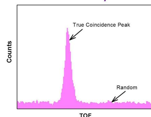
7- Events which correspond to real coincidences (true coincidence peak) were selected and a "playback" experiment can always be performed in the off-line analysis mode to examine the correlation between the charge-states of recoil ions and backscattered projectiles.
