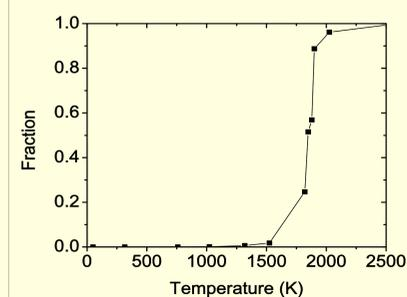
**Figure 3:** Fraction of Liquid-like atoms upon heating
