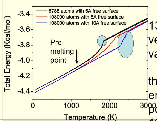
Melting point of model 13x13x13 is 1826K versus experimental value - 1728K.
